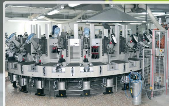
▲ 3 Desma units are installed at the Yoshkar-Ola Shoes Factory to fabricate shoes by the molded construction method
