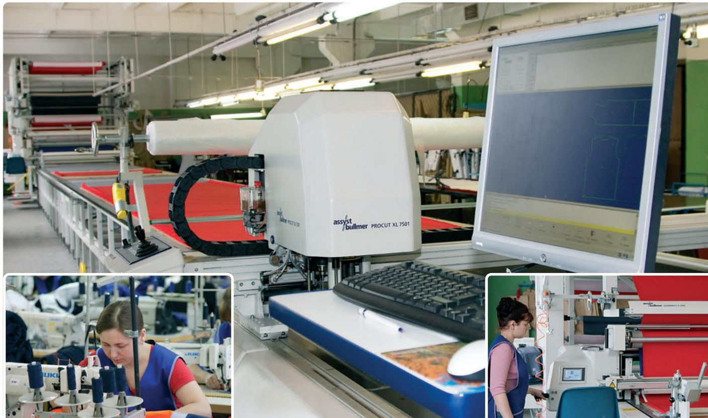
▲ Bullmer, automated cloth spreading and cutting complex at the Vyazma clothing factory
