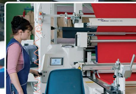
▲ Operator of the automated cloth spreading and cutting complex (ACSCC) at work
