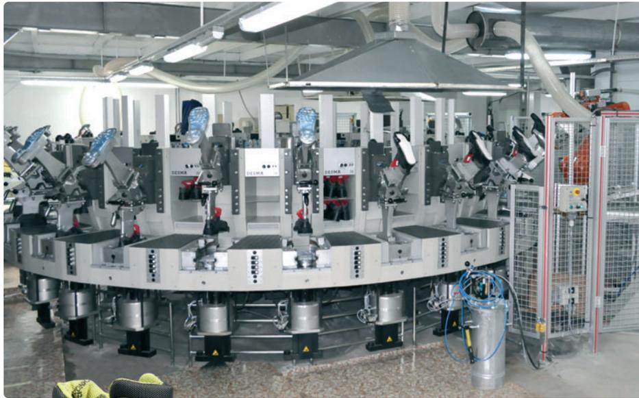
▲ New machines by Desma for fabricating shoes using direct sole attach construction method
