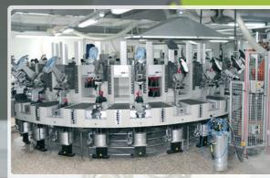
3 Desma units are installed at the Yoshkar-Ola Shoes Factory to fabricate shoes by the molded construction method
