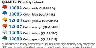
(PP) ventilated outer shell protects from head traumas caused by small falling objects. Polyamide harness lining has 3 textile bands with 8 fixing points and a foam sweat band. The helmet has 2 possible positions of the headband (top/low) for better comfort. This helmet can be used with accessories: JUGALPHA or DYNAMIC JUGALHPA MENTALPHA. Ratchet size adjustment: 53/63 cm. **Colors:** Blue, Green, Orange, Red, White, Yellow **Weight:** 360 g / 0.79 lbs. Adjustable ventilation shell **EN397**
